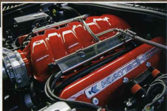
Top: Side profile on C6RS is clean yet purposeful sans excess appendages. Middle: The normally aspirated 8.2-liter Katech motor is machined out of a solid billet of aluminum. Bottom: Front profile showcases fender louvers and front splitter.
