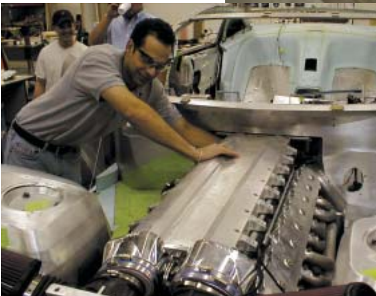
Test-fitting the engine in place.
