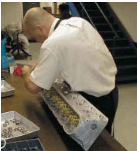
Valve spring installation.
